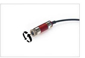
this case, the collimator assembly is first unscrewed relatively far, then screw varnish is applied to the thread and screwed back in to the appropriate focus. After the screw lacquer has dried, the optics is fixed.
